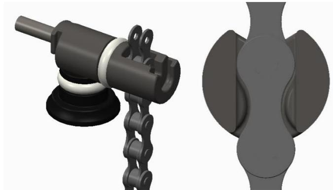
Wind the breaker screw in by hand until it contacts the chain rivet. You may need to adjust the chain position slightly to ensure the screw and rivet are aligned. You can now use your wrench to drive the breaker screw, pushing the rivet through the chain.
